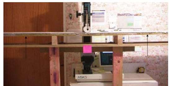
Particleboard floor under deflection, notice the 'S' bend occurring within the floor, with the central span bending in compression with the outer spans uplifting in tension.
